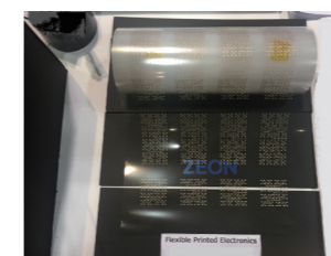
Using ZEONEX®C2420 in flexible substrate for millimeter-wave radar antenna
